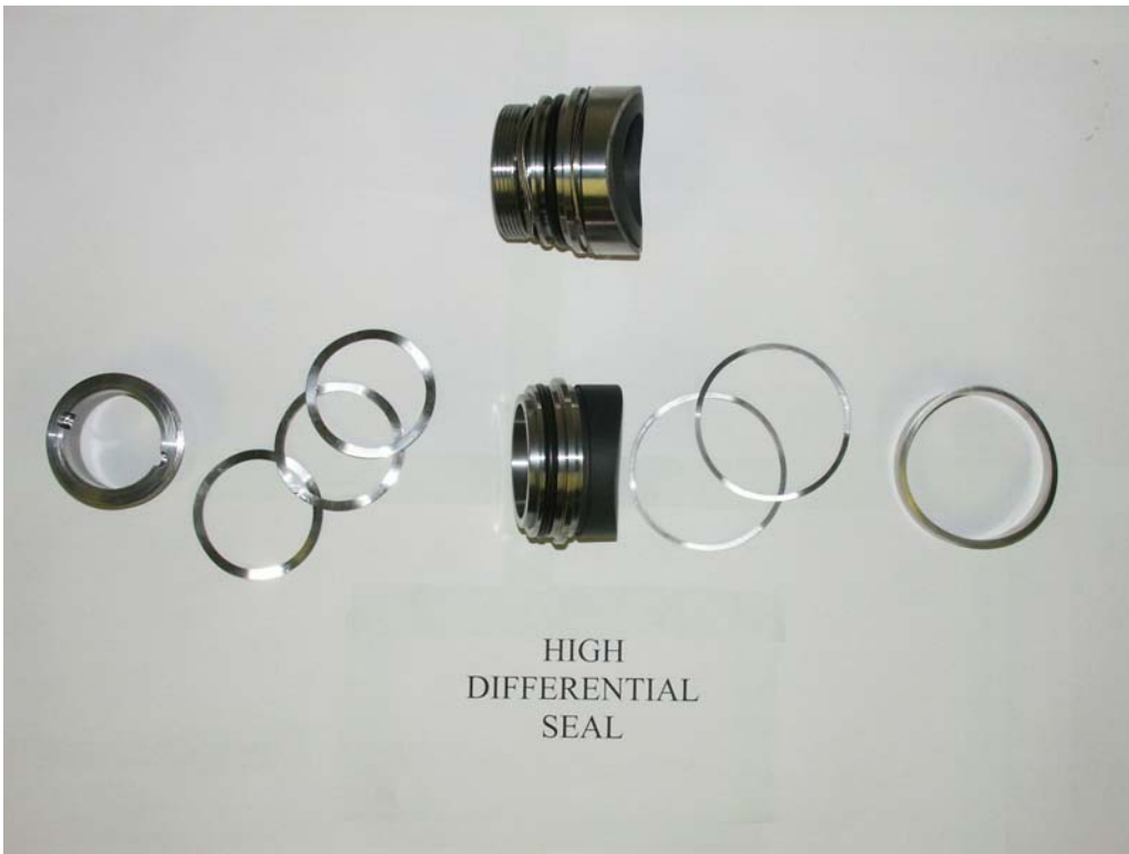
SEAL ASSEMBLY (TOP: ASSEMBLY. BOTTOM (L→R): SEAL ADJUSTMENT NUT, SEAL WAVE SPRINGS, SEAT RING/PLATE/O-RING/SEAL INSERT, SCRAPER WAVE SPRINGS, SCRAPER)
